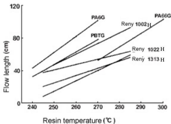
Figure 3. Temperature dependency of spiral flow (mold temperature 130 °C , injection pressure 98MPa)
