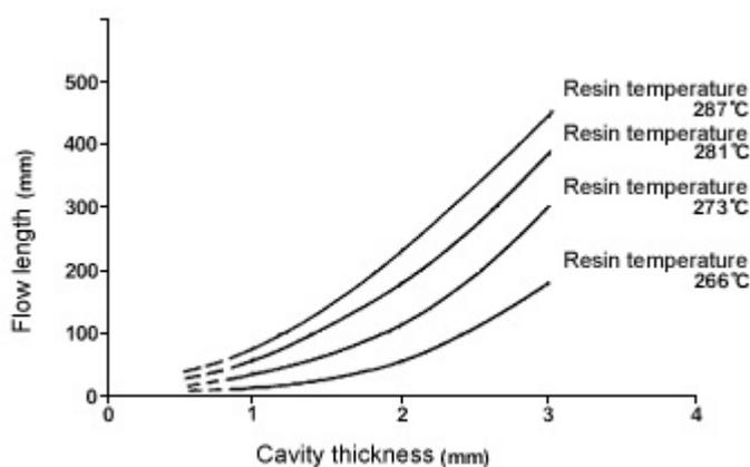
Figure 13. Cavity thickness and flow length of Reny1022 (gate diameter 1mm $\phi$ , injection pressure 109MPa, mold temperature 130°C)
