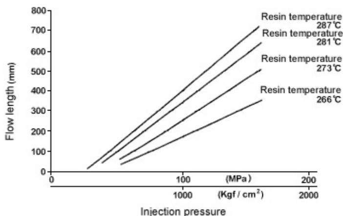
Figure 10. Pressure dependency of Reny1022 bar-flow (cavity thickness 3mm) (gate diameter 1mm $\phi$ , cavity thickness 3mm, mold temperature 130°C)
