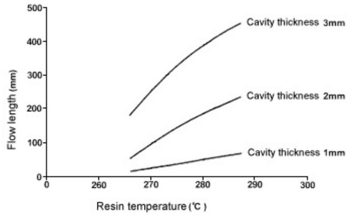
Figure 11. Resin temperature and flow length of Reny1022
