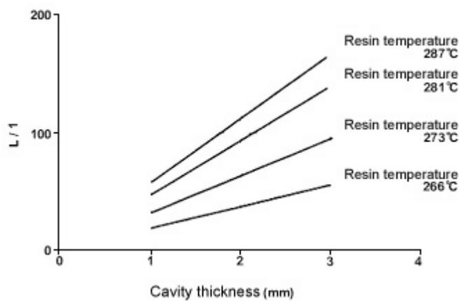
Figure 15. Cavity thickness and L/t of Reny1022 (gate diameter 1mmÖ, injection pressure 109MPa, mold temperature 130°C)
