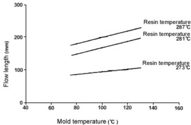
Figure 16. Mold temperature and flow length of Reny1022
