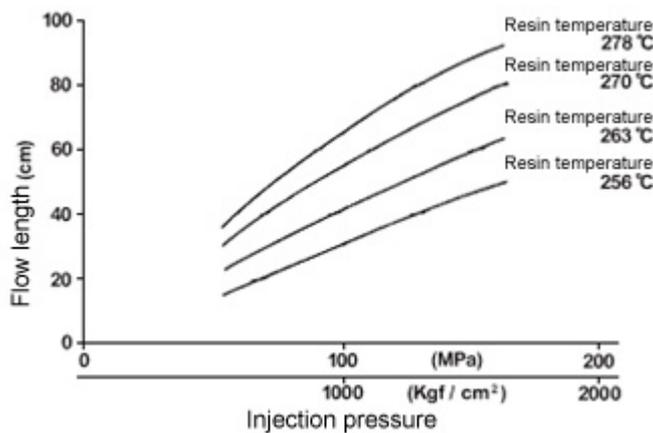
Figure 4. Pressure dependency of spiral flow of Reny1022 (mold temperature 130°C)
