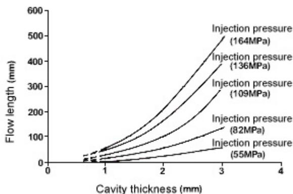
Figure 12. Cavity thickness and flow length of Reny1022 (gate diameter 1mm $\phi$ , resin temperature 273°C, mold temperature 130°C)
