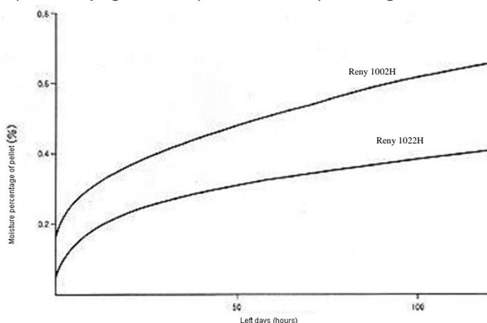
Figure 1. Relation of left time and pellet moisture percentage in 23°C, 55%RH
