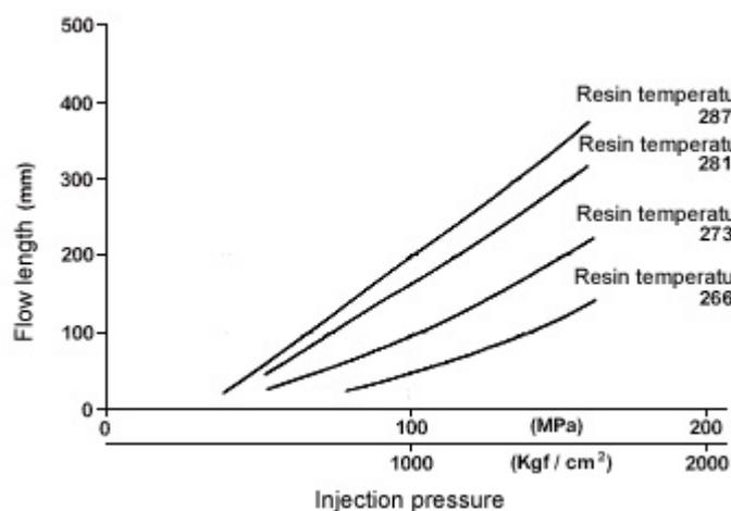
Figure 9. Pressure dependency of Reny1022 bar-flow (cavity thickness 2mm) (gate diameter 1mm $\phi$ , cavity thickness 2mm, mold temperature 130°C)
