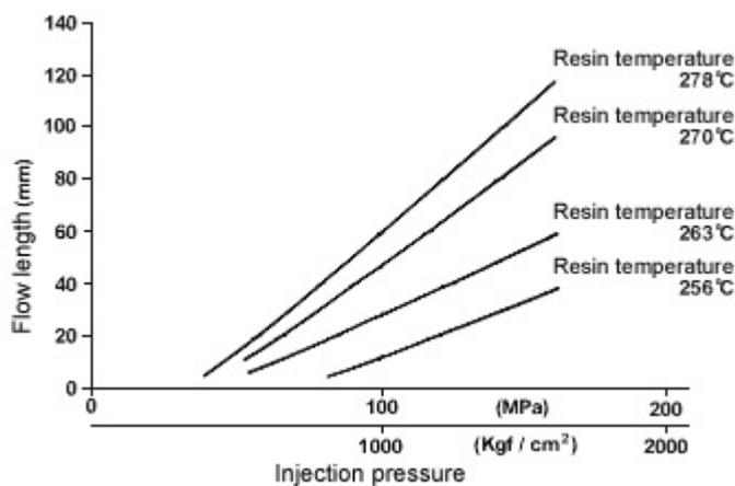
Figure 8. Pressure dependency of Reny1022 bar-flow (cavity thickness 1mm) (gate diameter 1mm $\phi$ , cavity thickness 1mm, resin temperature 130°C)
