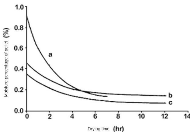
Figure 2 Pellet drying time and moisture percentage
